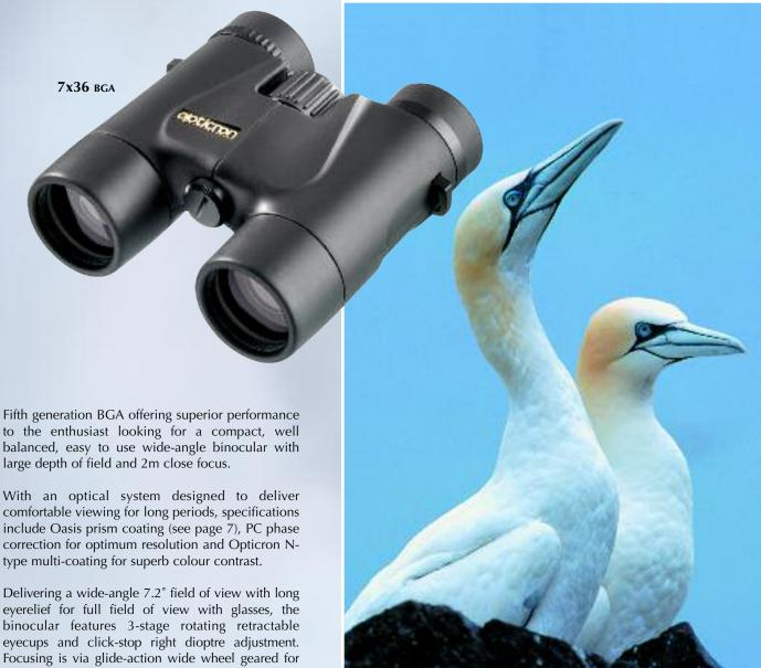
eyerelief for full field of view with glasses, the binocular features 3-stage rotating retractable eyecups and click-stop right dioptre adjustment. Focusing is via glide-action wide wheel geared for 540° or 1.5 turn from 2 metres to infinity.
