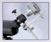
Many digital compact cameras do not have screw threads on the lens housing to allow for direct coupling, so the UDCA is designed as a three-way adjustable balance plate that fixes directly to the telescope eyepiece. The camera is fixed onto the UDCA and can be adjusted on three planes to enable correct positioning with respect to the eyepiece.
