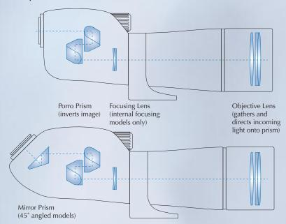
**Specifications** Opticron telescopes are generally supplied in 'body only' format e.g. MM2 52, HR 66, ES 80. These models have objective lens diameters of 52mm, 66mm and 80mm respectively, no built-in eyepiece and as such allow the choice of eyepiece to be made separately.
