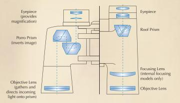
**Z** or **B** stand for **porro prism** binoculars. The basic optical design of these 'traditional-shape' instruments mean they tend to deliver better optical performance for your money compared to **roof prism** (**D**) binoculars, which are more compact but also more expensive.
